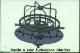
Inside a Low Turbulence Clarifier
