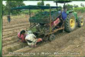
Planting using a Water-Wheel Planter
